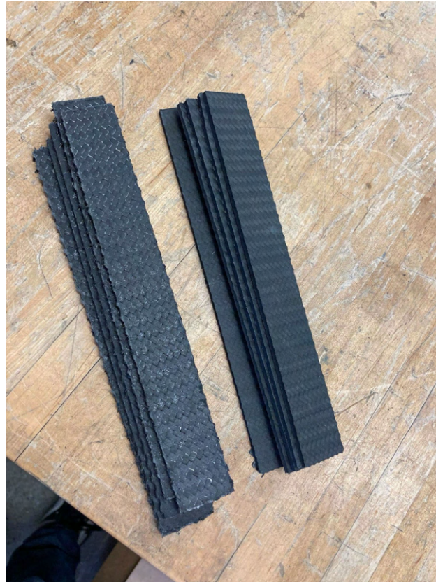
Figure 45: Fin Plate Testing Samples - SRAD (right) and COTS (left)
