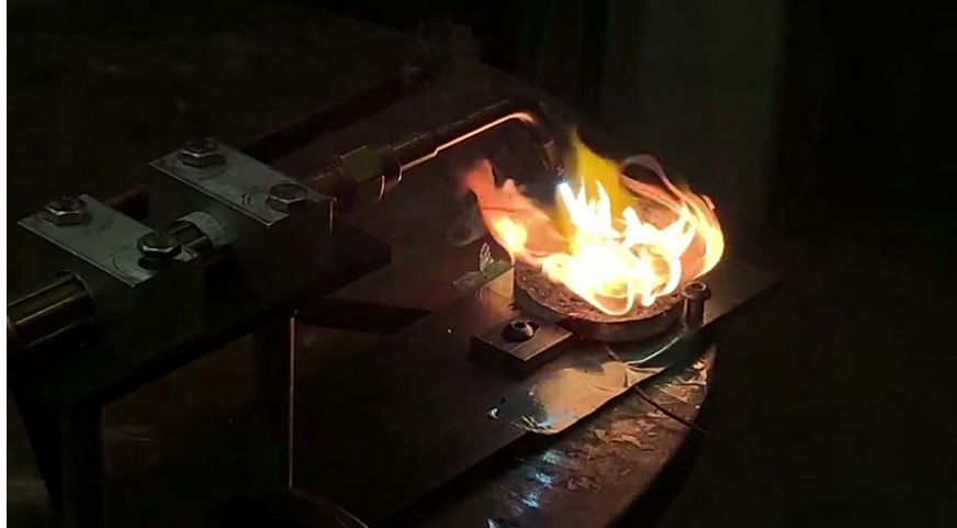
Figure 64: Ablative Characterization Testing Setup and Test
