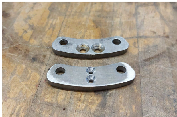
Figure 35: Screw Layout of Curved Tabs - 2024 (Bottom) and 2023 (Top)
