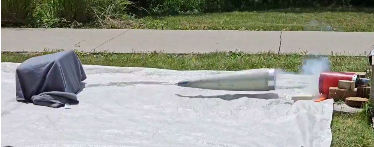
Figure 99: Deployment test completed to verify new o-ring seal integrity with this year's flight components
