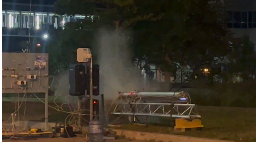
Figure 164: Nitrogen and Water Being Sent Through the Injector Valves During WDR 1
