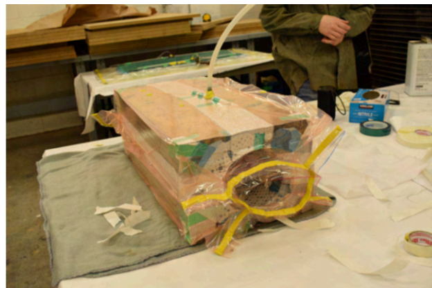
Figure 23: Nosecone Curing Under Vacuum
