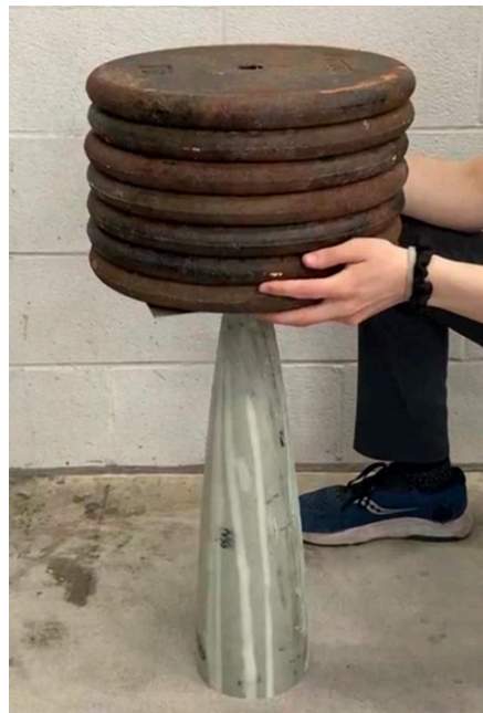
Figure 24: Nosecone Compression Testing
