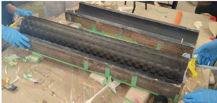
Figure 27: Fin Can and Combustion Chamber Bodytube Demoulding
