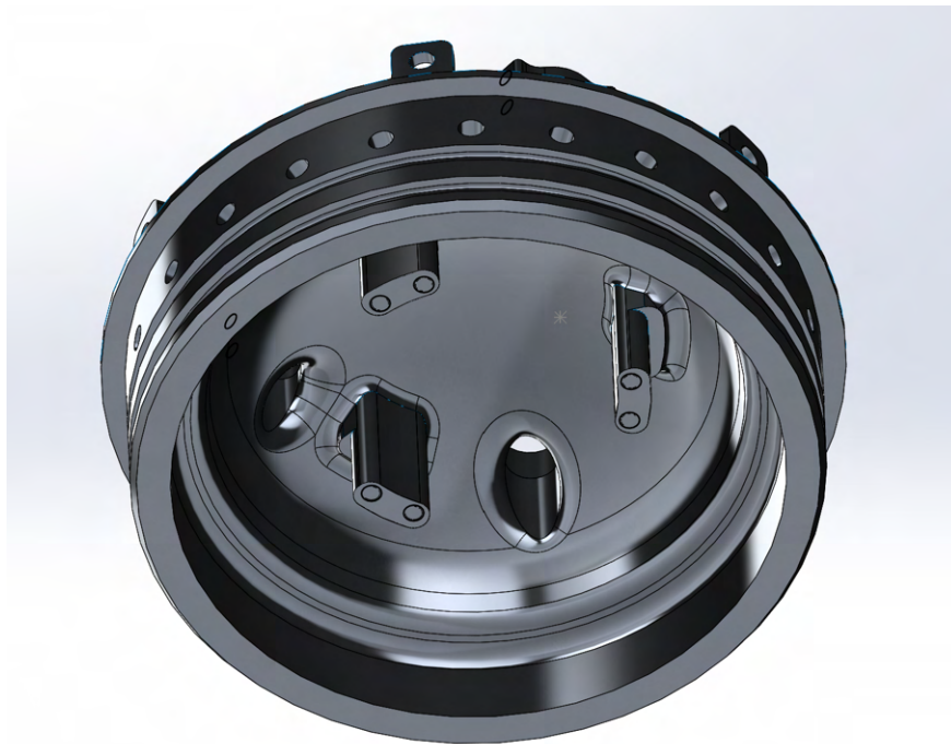
Figure 68: Centering Features of Vent Bulkhead
