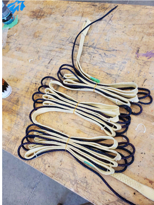
Figure 101: Routed and Folded Reefing Wire and Shock Cord Bundles
