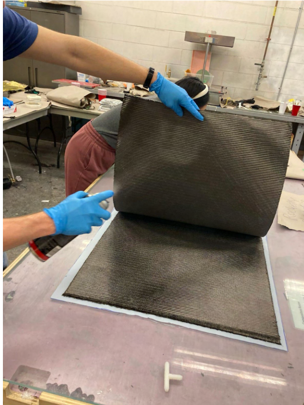
Figure 49: Plate Layer Assembly
