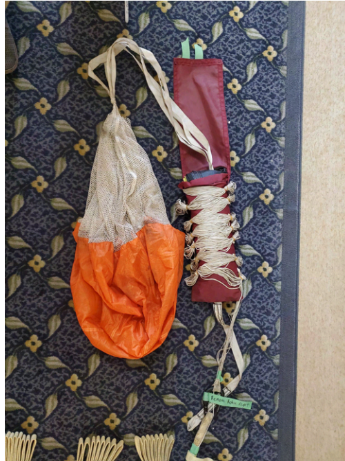
Figure 103: Packed Parachute and Rigging
