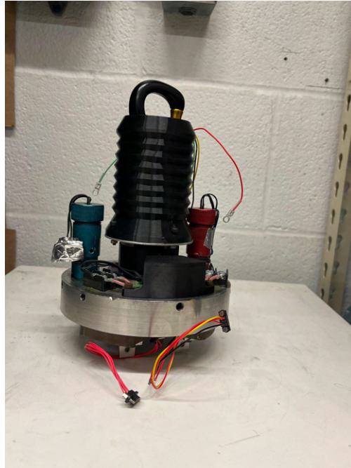
Figure 102: Integrated Recovery Bulkhead with Slipping Shroud
