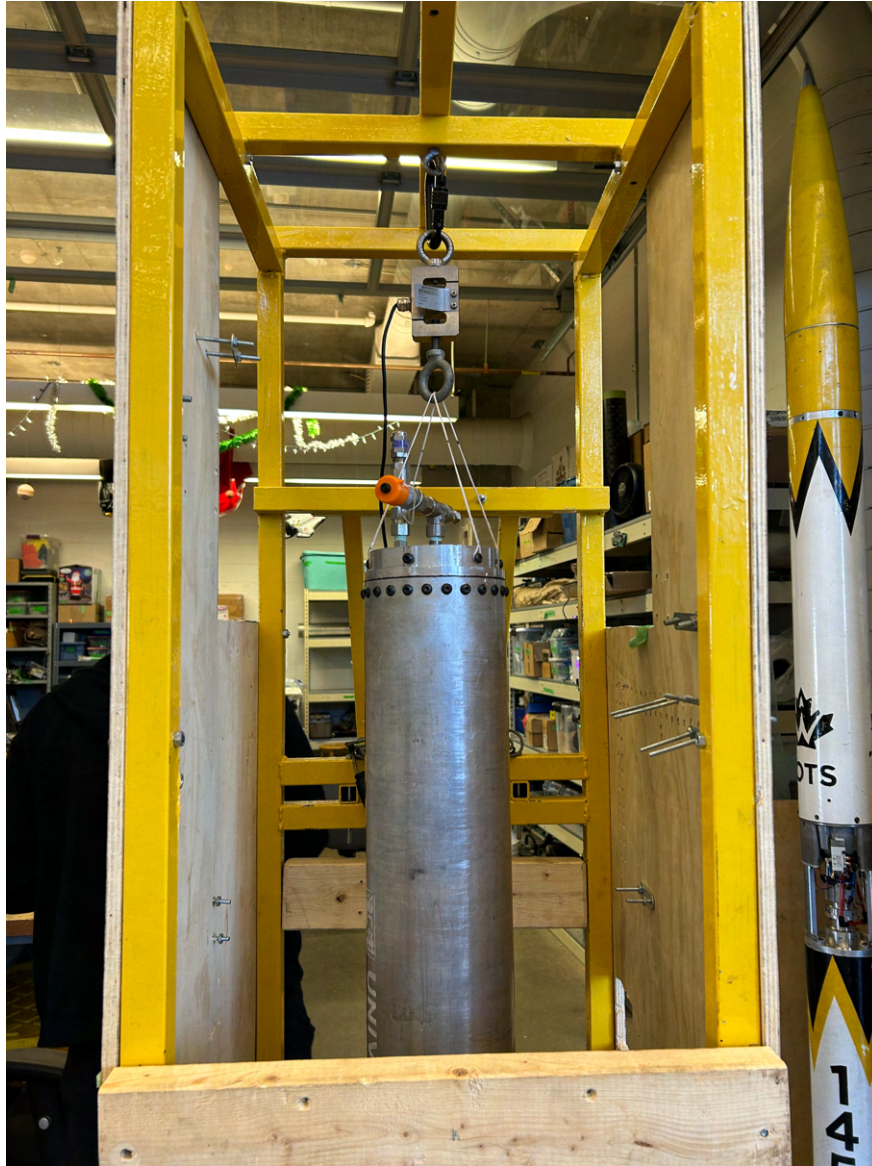
Figure 57: Cold Flow Test Load Cell Set-up
