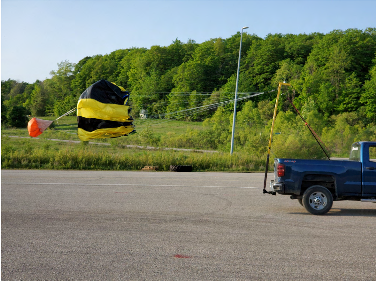
Figure 98: Truck Testing a Previous Year's Parachute
