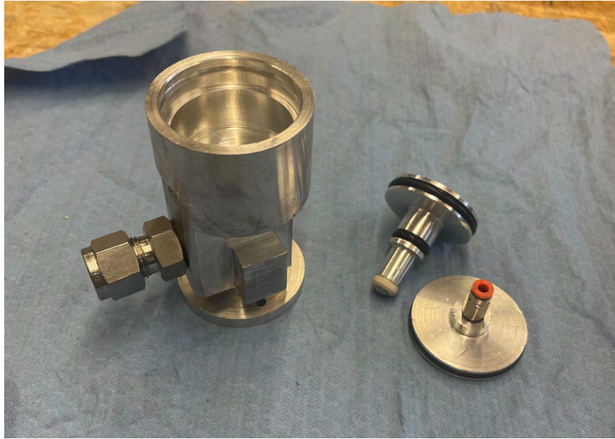
Figure 77: Finished Fill/Dump Valve
