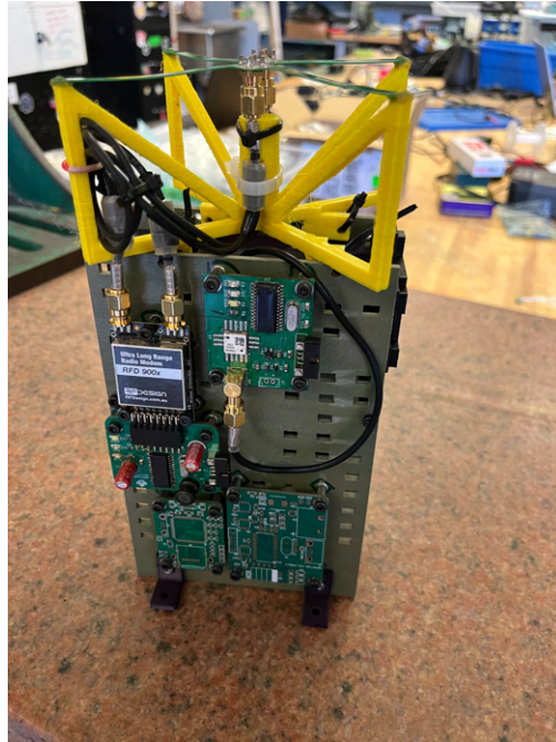
Figure 100: Recovery Electronics Sled
