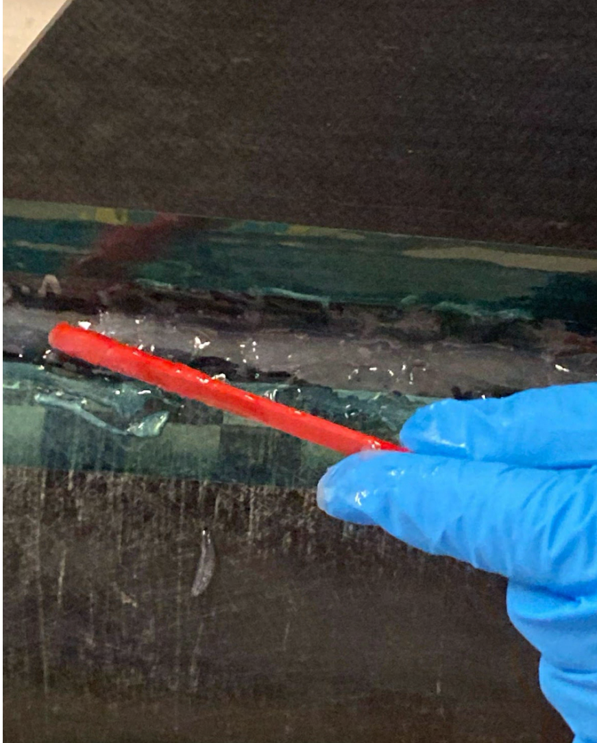
Figure 39: Fillet Being Formed Using Popsicle Stick
