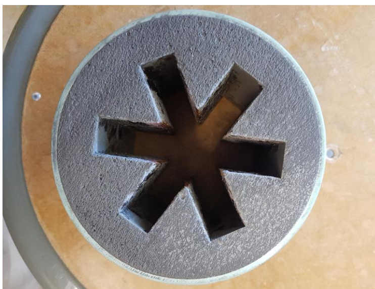
Figure 4. Kismet fuel grain. The parameters for the pseudo-finocyl grain geometry were empirically determined by the team through numerous static fires.
