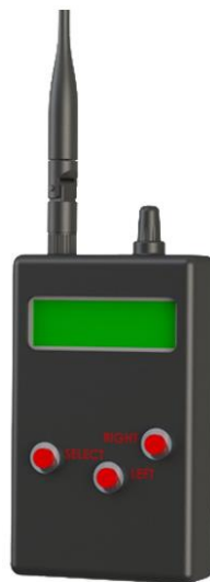
Figure 12. Payload transponder. The antenna for the radio transceiver, LCD, navigation buttons, and potentiometer for LCD contrast are visible.
