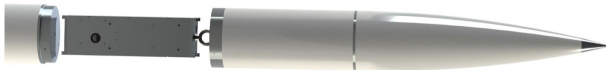
Figure 10. Render of complete payload system. The CubeSat can be seen at the left of the image. Also visible is the deployment mount (center; airframe tube) and the nose cone.
