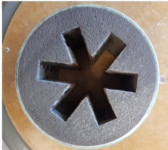
Figure 7. Cross-section of the Kismet fuel grain.
