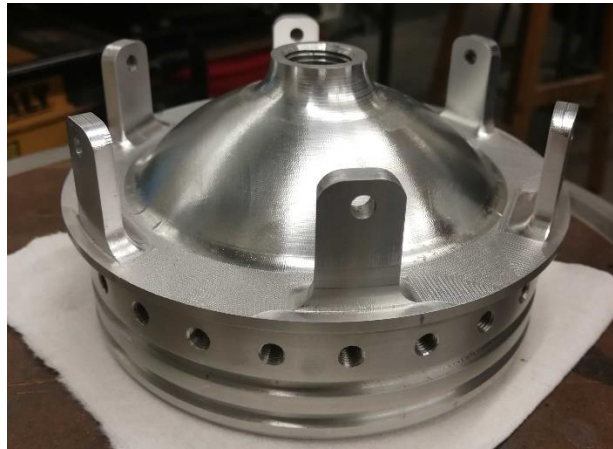
Figure 3. Oxidizer tank fill bulkhead.
