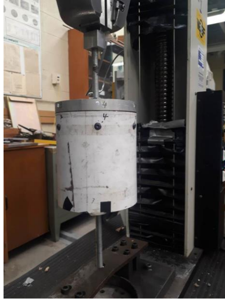
Figure 10. Tensile test of fibreglass-aluminium coupling.
